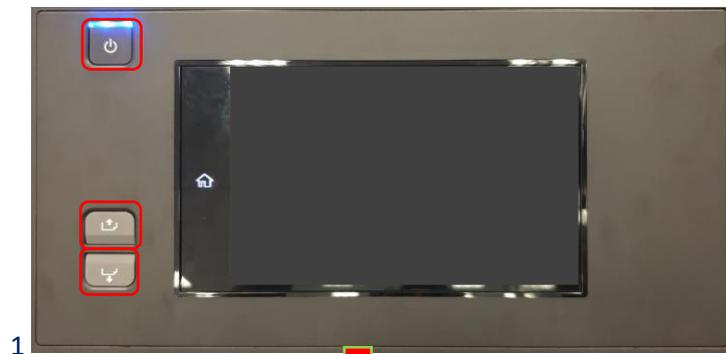
In "OFF" mode, Press and hold the three buttons highlighted in red (hold down for 25 seconds or more) to activate User Self Repair Mode!
